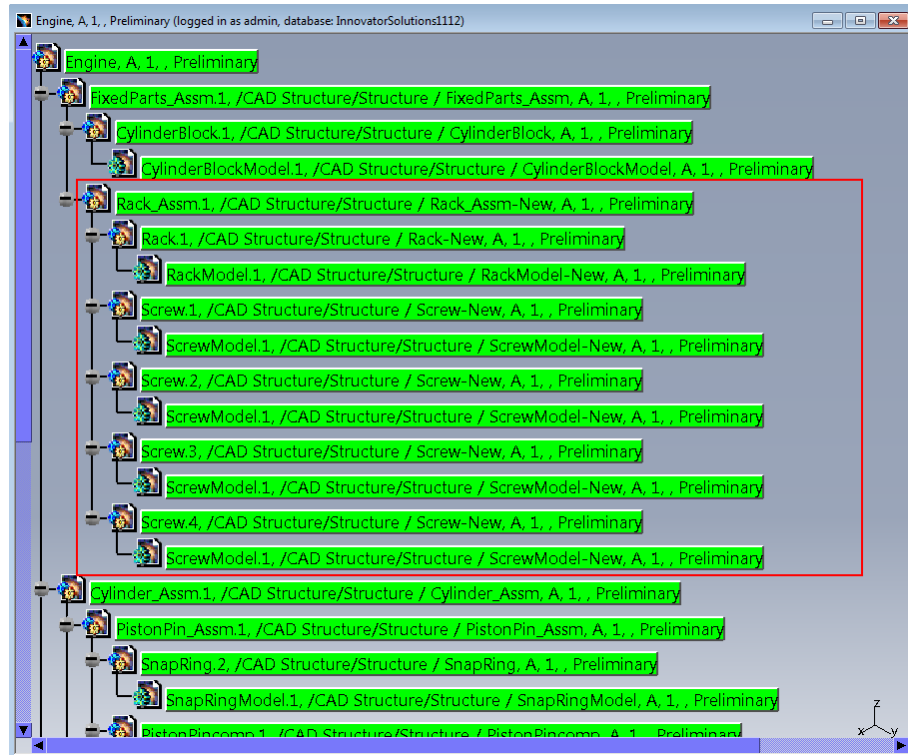
Picture 132: Existing PDM structure containing new substructure
